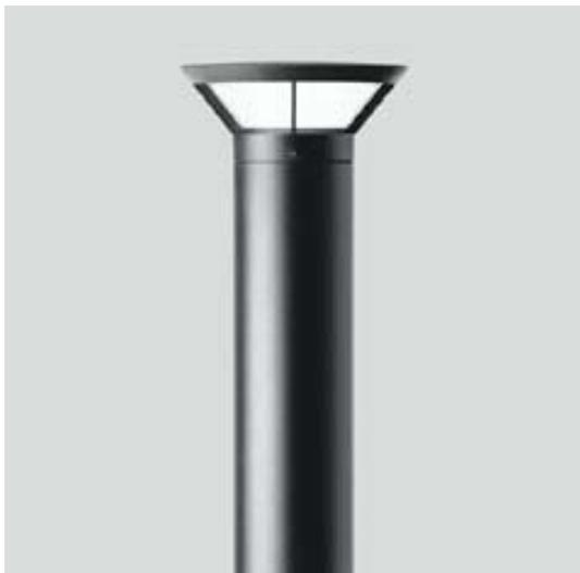
BEGA-8543 Bollard with shielded light source for 1 discharge lamp HIT-CE 35 W, socket G 12, 3.400 lumen. Protection class IP 65.
