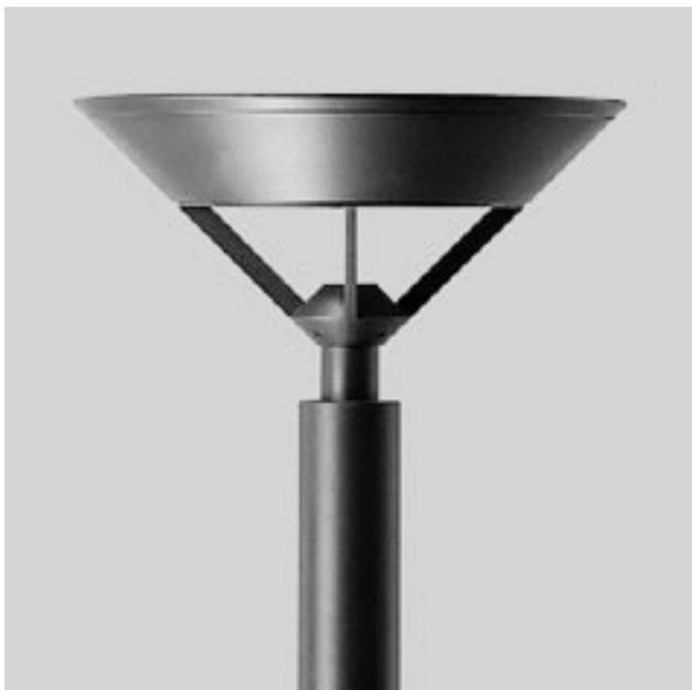
BEGA-8081 Pole-top luminaire with symmetrical light distribution for 1 discharge lamp HME-50W, 1.8 Klm. Protection class IP 44. Aluminium alloy, aluminium and stainless steel. Clear safety glass. Reflector of anodized pure aluminium. Luminaire with fixed connecting cable H05VV-F 3 x 1 sqmm. Cable length: 9.000 mm. The luminaire is designed for the pole heights: 3.000 mm. Pole top  $\varnothing$  76 mm · Insert depth 100 mm. Colour: graphite - article number silver - article number + A
