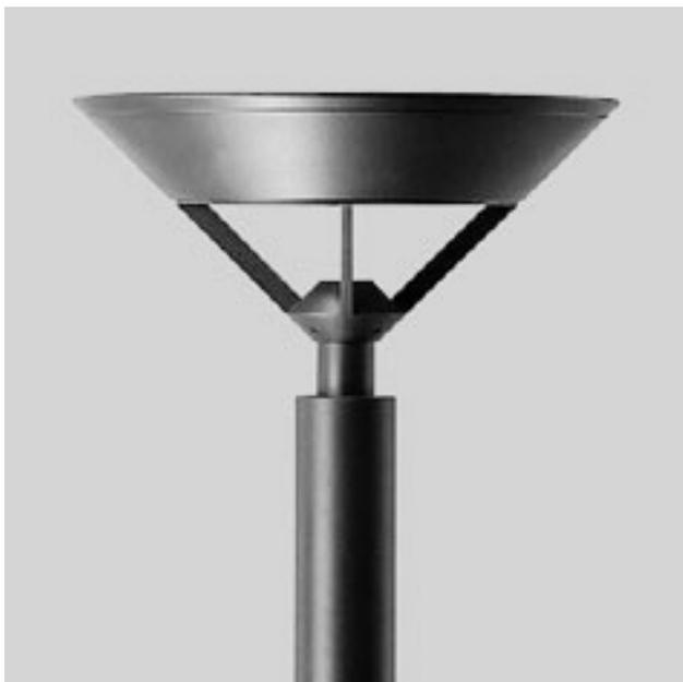
BEGA-8086 Pole-top luminaire with symmetrical light distribution for 1 discharge lamp HIE-250 W, 17.000 lumen. Protection class IP 44. Aluminium alloy, aluminium and stainless steel. Clear safety glass. Reflector of anodized pure aluminium. Luminaire with fixed connecting cable H05VV-F 3 x 1 sqmm. Cable length: 9.000 mm. The luminaire is designed for the pole heights: 9.000 mm. Pole top  $\varnothing$  76 mm · Insert depth 100 mm. Colour: graphite - article number silver - article number + A
